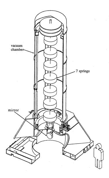
Figure 2: Front view of the super-attenuator.
