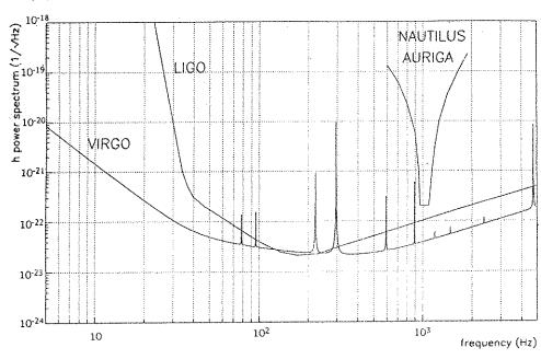
Fig.3 – Expected sensitivities of VIRGO and LIGO expressed as the linear spectral densities of the dimensionless amplitudes of the noise  $(\tilde{h}(f))$ .
