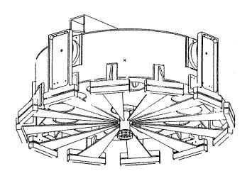
Figure 3: View of a single filter of the super-attenuator. The triangular blade springs which provide the vertical attenuation are visible.
