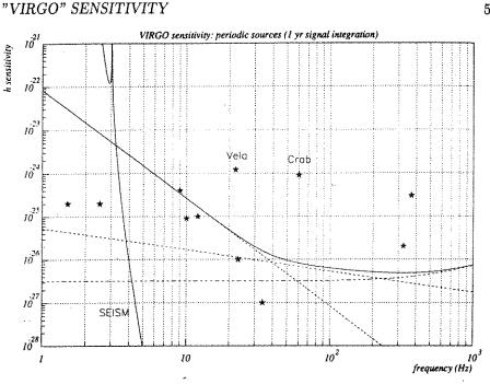
Figure 4: VIRGO h sensitivity to periodic sources (1 yr signal integration). Notice that the seismic noise dominates at very low frequencies, but it is "cut" for f < 4Hz: this clearly illustrates the action of the super-attenuator. The dashed lines represent the suspension thermal noise (which dominates at 4 < f < 40 Hz), the mirror thermal noise (40 < f < 200 Hz), and the laser shot noise (f > 200 Hz). The "stars" mark the expected  $h_{max}$  of the pulsars listed in the Table.
